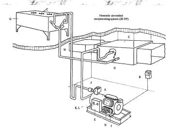
compressor break down. If you see signs of wear or fatigue, replace them. (Valves are relatively inexpensive.) AVOID LUBRICATION FAILURE.
